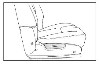
Lift the recliner lever, located on the outboard side of the seat, up fully and fold the seatback forward until it disengages.
